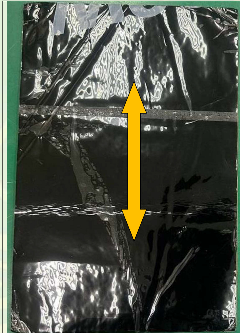
Test specimen orientation for testing (Vertical Direction)
